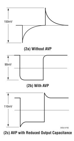
Figure 2. Transient Response Comparison
