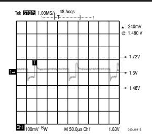
Figure 12. LTC1703 Transient Response with AVP – 4 Output Capacitors with Load Step from OA to 14A
