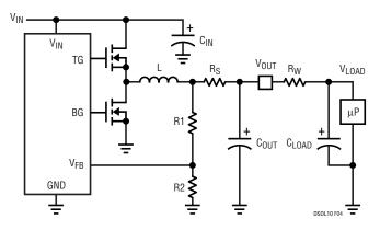
Figure 4. Simplified Buck Regulator with Current Sense Resistor and Wiring Resistance
