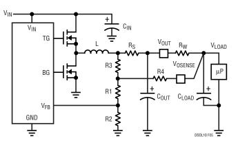
Figure 5. Simplified Buck Regulator with Remote Sense
